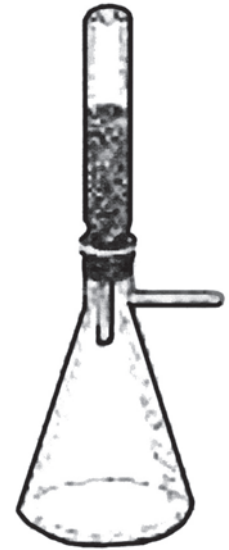
Tswett's chromatography apparatus, 1903
